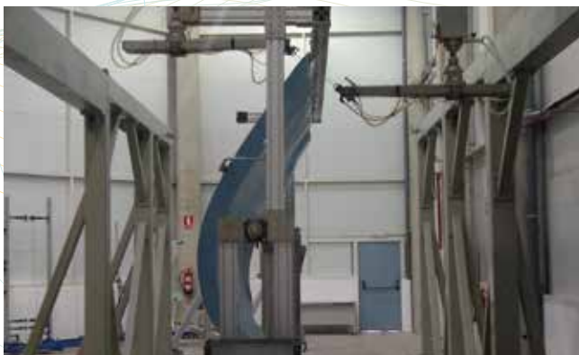
Travelling bridges scanner
