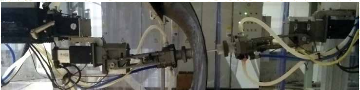
Dual tower scanner with mobile immersion tank
