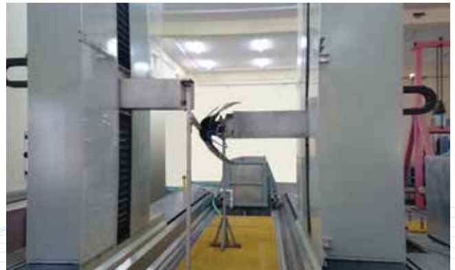
Dual tower scanner with mobile immersion tank
